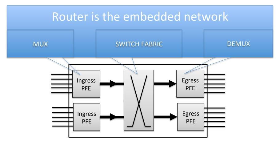
PFE – a CPU, NPU or ASIC that process packet
