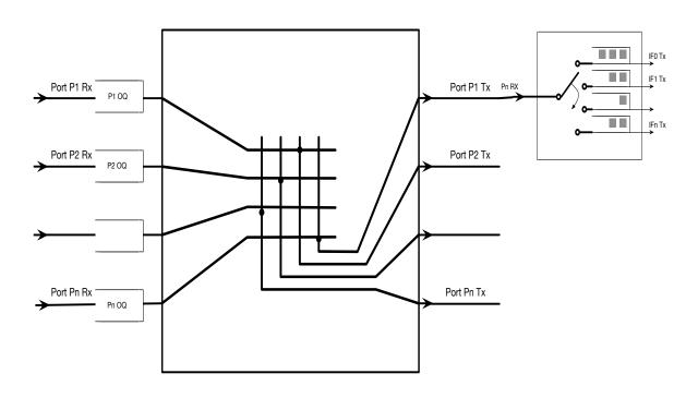
IQ requairments for loss-less: Fabric Port speed >>  $\Sigma$  (ASIC egress interfaces)
