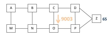
A packet injected at node C with active segment 9003 is forced through datalink CO
