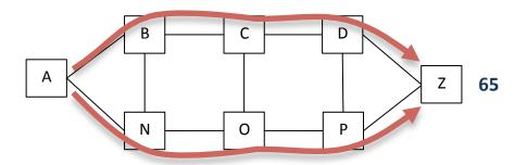
A packet injected anywhere with active segment 65 will reach Z via ecmp-aware shortest-path
