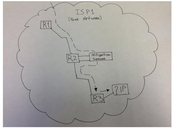
In-line mitigation for an environment running a low traffic application
