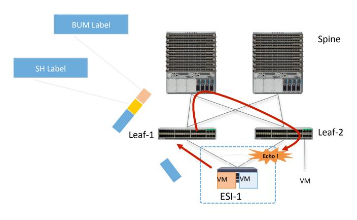
Per- ESI SHG Label EXT-COMM with EVPN RT-1 enables SHG filtering to cut potential loops back to same ESI
