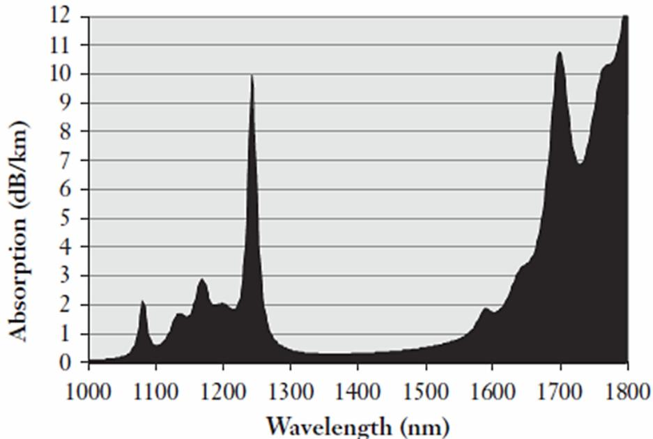
Attenuation of Standard vs. Low Water Peak Fiber
