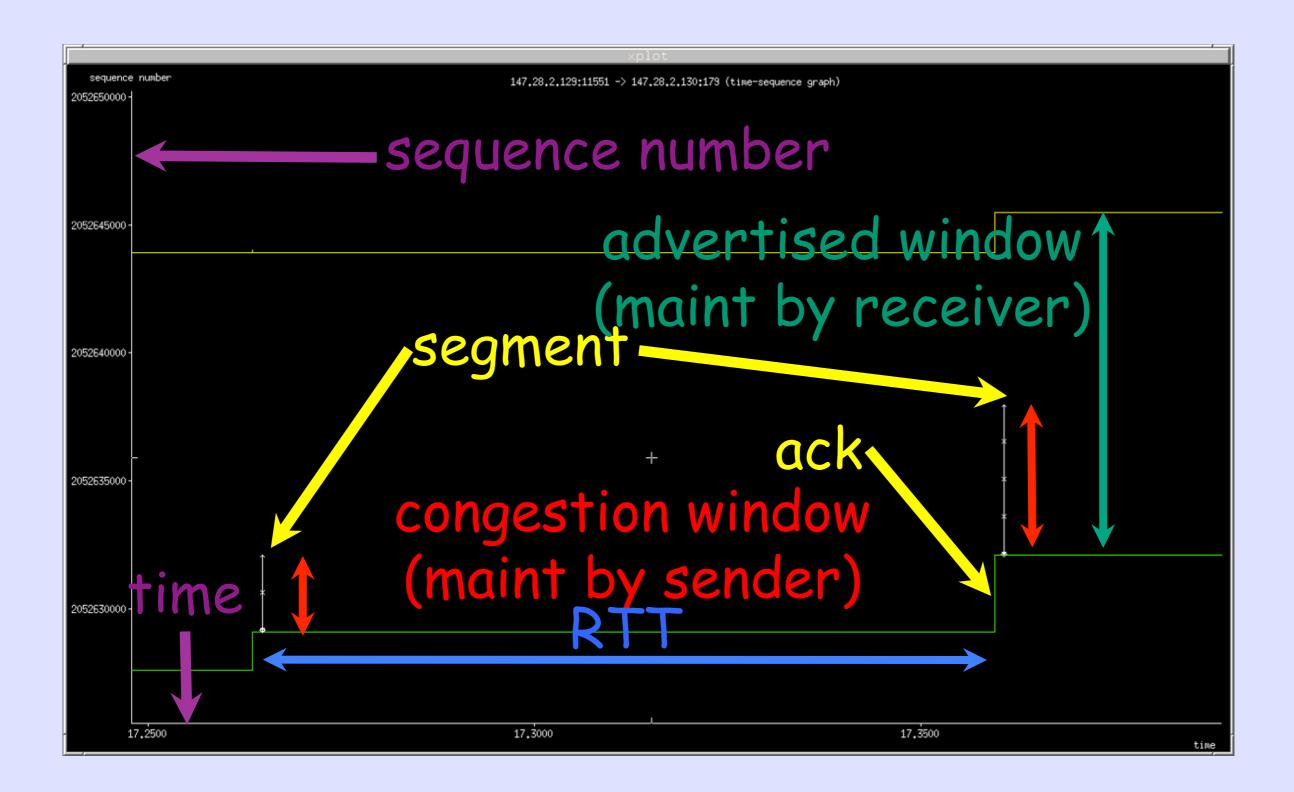
Warning: In xplot, relative scaling of axes is completely arbitrary, i.e., one can zoom one without the other and often does by accident.
