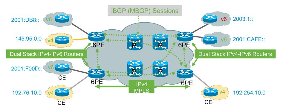
IPv6 global connectivity over and IPv4-MPLS core
