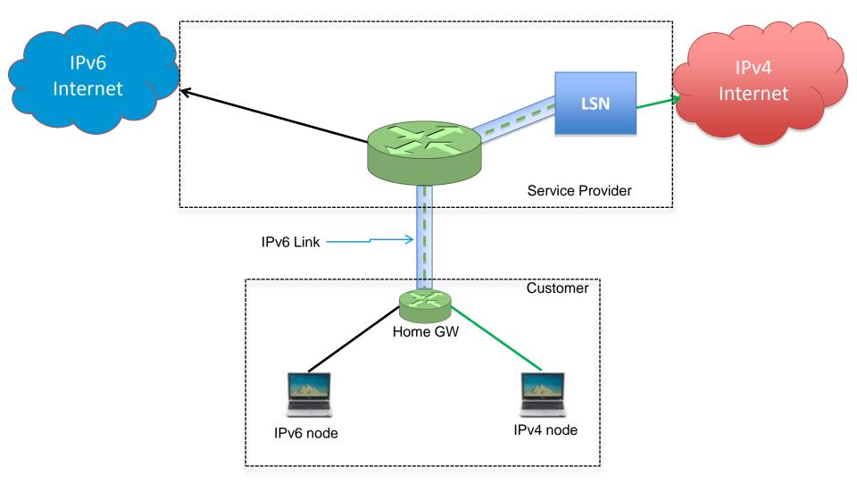
IPv6 packets are routed normally, while IPv4 packets are encapsulated in IPv6 and routed to the LSN
