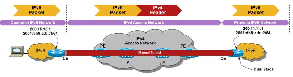
One of the first transition mechanisms developed for IPv6
