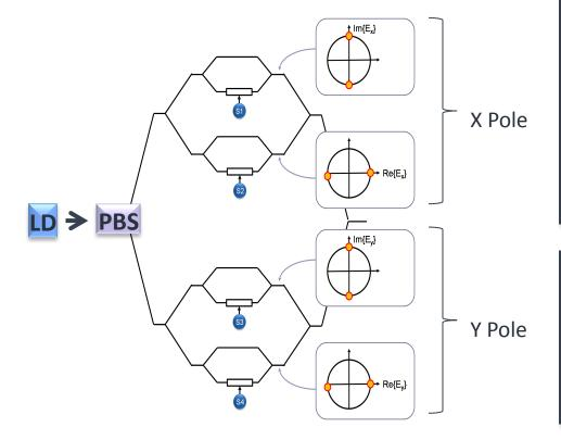
If built with discrete optical components, it would be logical to economize, and build separate boards for PM-QPSK & PM-BPSK
