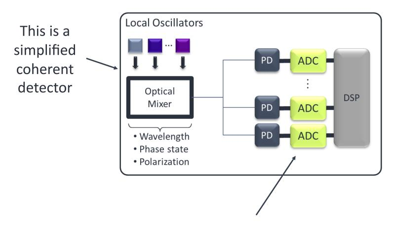
Coherent detection requires very high speed Analog to Digital Converters
