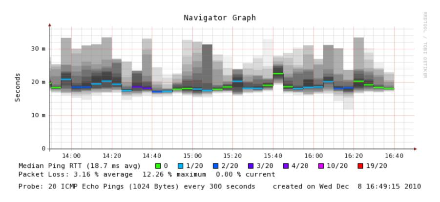
QOS knobs in router set empirically - stable latency at all loads From > 1 second, to less than 10 milliseconds jitter and latency - 100 times better!
