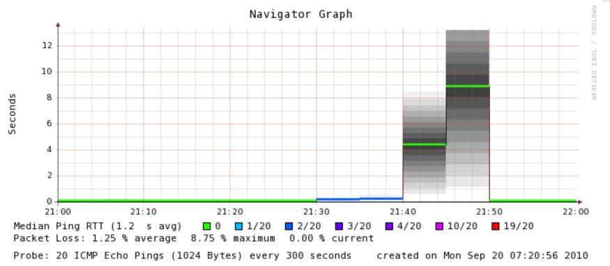
8 second latency over a path of less than 10ms! Much worse than my broadband only test
