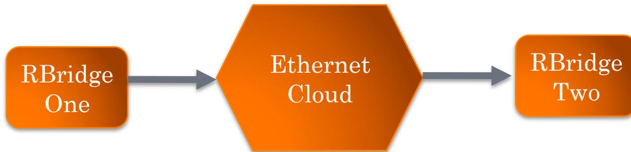
\* Link Transport VLAN need only be present if RBridges are connected by a bridged LAN or carrier Ethernet requiring a VLAN tag or the like.
