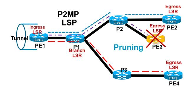
The operation of removing Egress LSRs from an existing P2MP LSP is termed **PRUNING**
