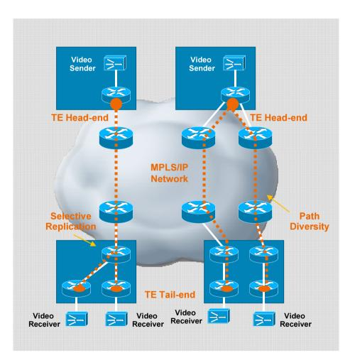
An typical P2MP TE Deployment for the Video distribution
