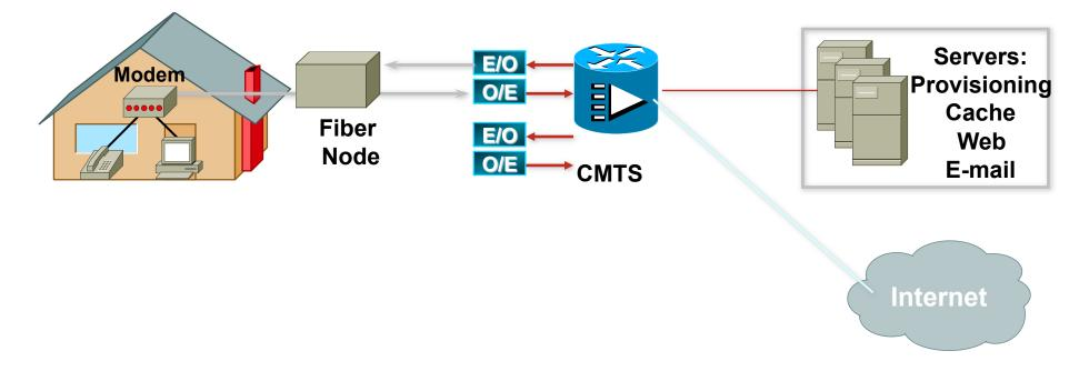
Note: E/O and O/E refer to the Electrical to Optical conversion of the signals in a cable HFC system
