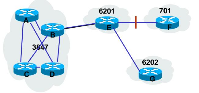
The following configuration could be used on router B to accept routes from AS6201 & 6202 and deny all others.
