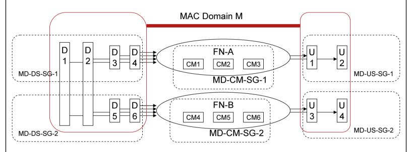
A MAC Domain Downstream Service Group (MD-DS-SG) is the set of downstream channels from a single MAC Domain that reach a single CM.
