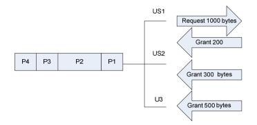
The CM has a buffer with a 1000 bytes to send. Its requests for 1000 on US1, the CM receives grants on US1, US2 and US3. The size of the grant may depend on the load on that channel
