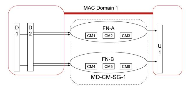
Usually, each fiber node is served by a unique set of upstream channels, and each MD-CM-SG corresponds to a single fiber node.
