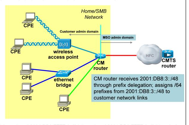
HFC link; assigned 2001:DB8:FFFF:0::/64 (mgmt) and 2001:DB8:FFFE:0::/64 (service)
