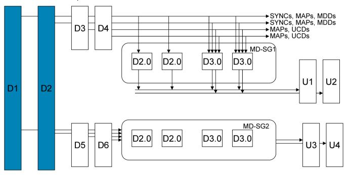
Primary Channel of a CM is the DS channel on which it receives SYNCs. Primary Capable Channel of a CMTS is a DS channel configured to send SYNCs. D1 and D2 in this figure.
