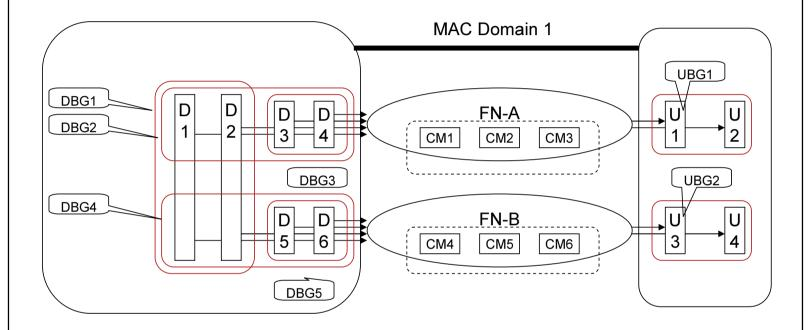
A downstream bonding group (DBG) is a set of channels on which the CMTS distributes a sequence of packets to a set of CMs;
