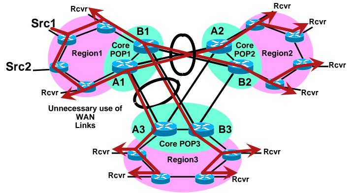
The same metric good for unicast load splitting cause multicast traffic to go unnecessarily across both the A and B WAN links.
