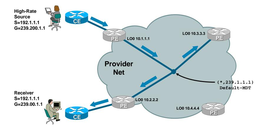
Traffic exceeds Data-MDT threshold configured on PE router
