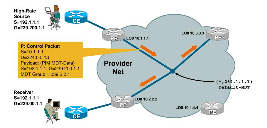
PE router signals switch to Data-MDT using new group, 239.2.2.1
