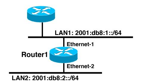
Dual IPv4/IPv6 configuration.
