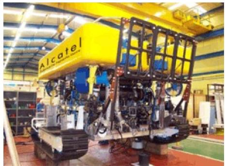
Burial capability, Work to 2500m, Most Cables now trenched offshore where permitted, Pre/Post Lay Inspections
