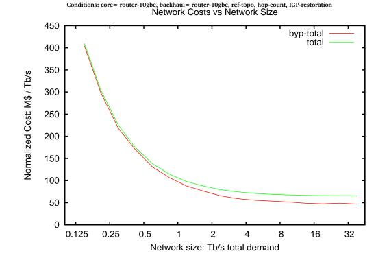
The cost per bit using router 10GbE with no bypass is compared to the cost per bit of applying bypass links until no further gain is possible.
