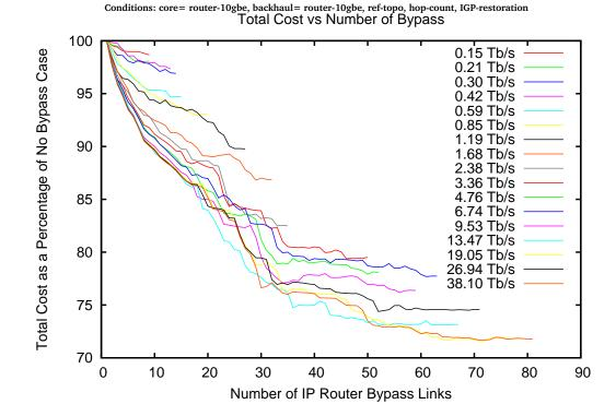
Software applies the bypass link which most reduces the number of router interface and iterates until no further reduction is possible.
