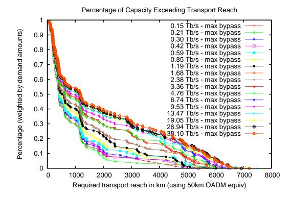
At small scale little or no bypass is used, therefore there is no impact on reach requirements.
