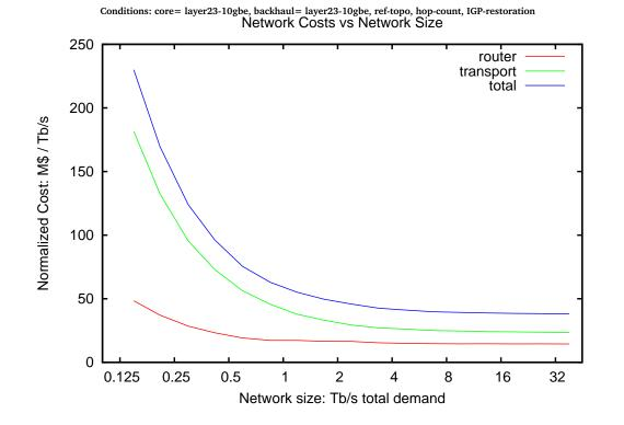
If the largest layer-2/3 switches are used in place of larger router and arranged in a CLOS, the router cost is reduced substantially.
