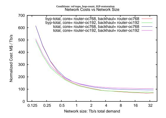
IP router bypass gives OC-192 a slight cost advantage over OC-768 within a range where 10Gb/s provides more opportunity for bypass than 40 Gb/s
