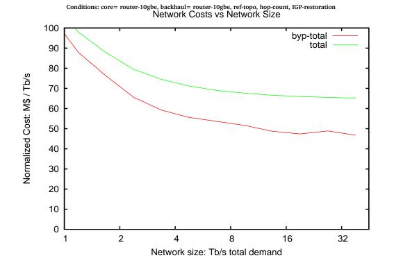
Total cost per bit of using no bypass and using maximum bypass are shown for large scale only.
