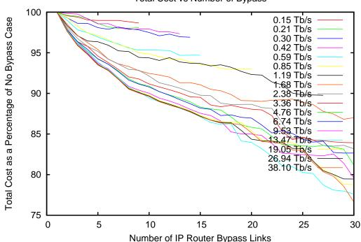
Conditions: core= router-10gbe, backhaul= router-10gbe, ref-topo, hop-count, IGP-restoration Total Cost vs Number of Bypass In this plot the X-axis is constrained to 30 bypass links.
