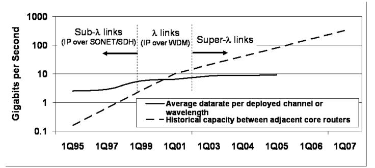
Bandwidth requirements strongly favors approach leveraging multiple wavelengths (aka Super-λ service, composite links, LAGs, etc.)
