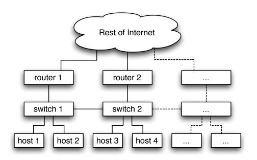
Routers and hosts communicate within a common subnet (e.g. a VLAN plumbed through some switches)
