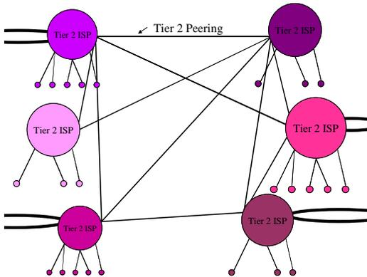
**Figure 8 – Generalized Tier 2 Interconnection Model**
