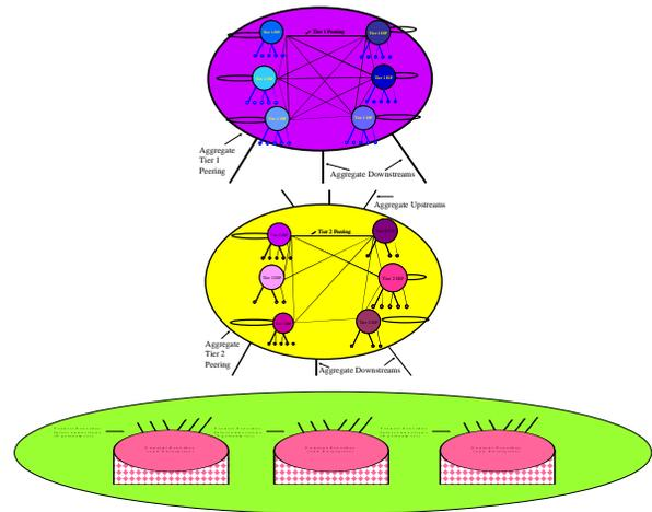
**Figure 11 - Tier 1 ISPs, Tier 2 ISPs, and Content Providers in the Peering Ecosystem**
