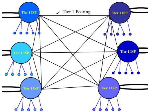
**Figure 3 - Generalized Tier 1 Interconnection Model**
