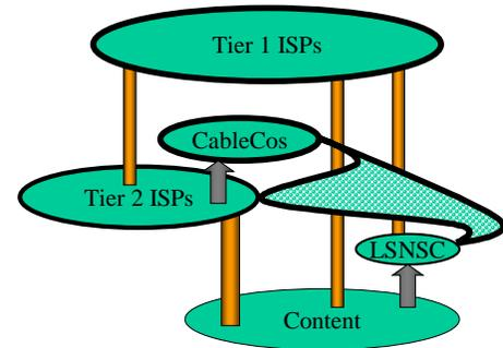
Figure 18 – Evolution #3 : Cable Companies peer with Large Scale Network Savvy Content Providers
