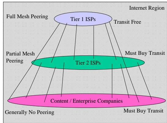
**Figure 10 - Generalized Peering Ecosystem, consisting of Tier 1 ISPs, Tier 2 ISPs, and Content/Enterprise Players.**
