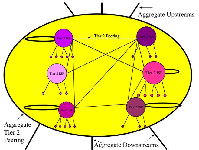
**Figure 9 - The Grouping of Tier 2 ISPs in the Peering Ecosystem.**
