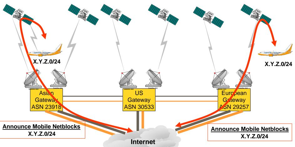
Commercial passenger traffic is released at each Ground Station. Each Ground Station only advertises the IP's for the planes it is serving. When a plane leaves a region, that gateway stops advertising its IP's.
