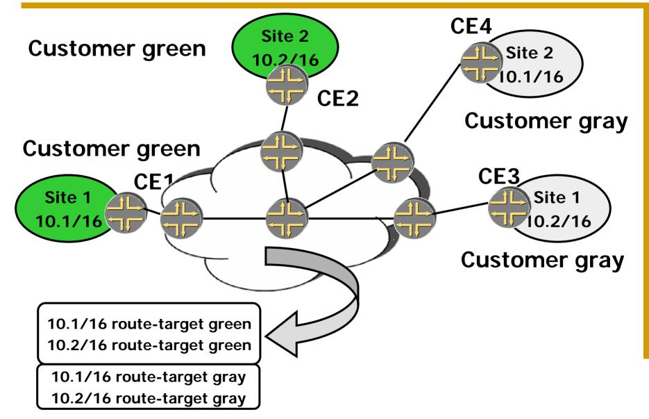
The P routers carry all VPN routes, so the addresses used in the VPNs need to be unique in the provider's network.
