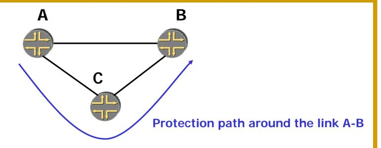
Will still have traffic loss: the failure needs to be detected, the traffic needs to be switched to the alternate path.
