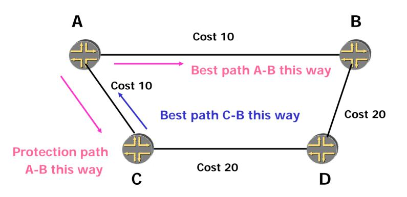
Goal – protect against failure of the link A-B
