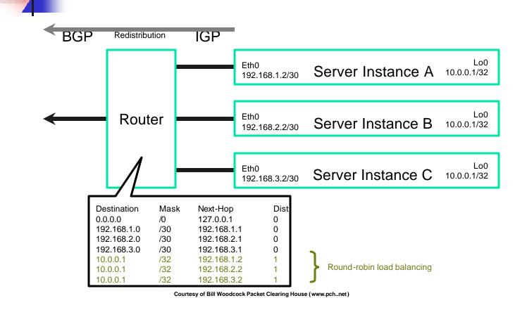
Two IP Addresses: One address for management & One address for anycasting.
