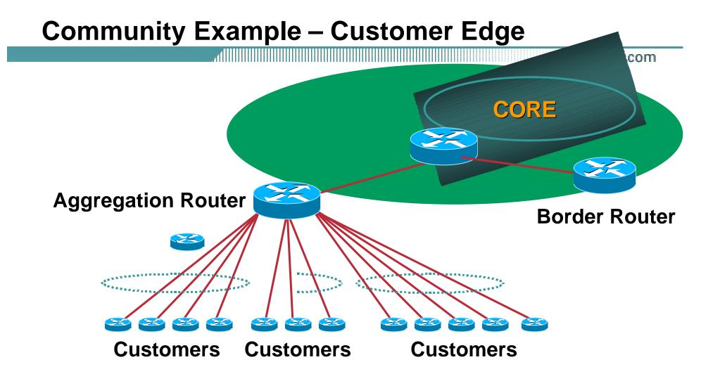
Communities set at the aggregation router where the prefix is injected into the ISP's iBGP
